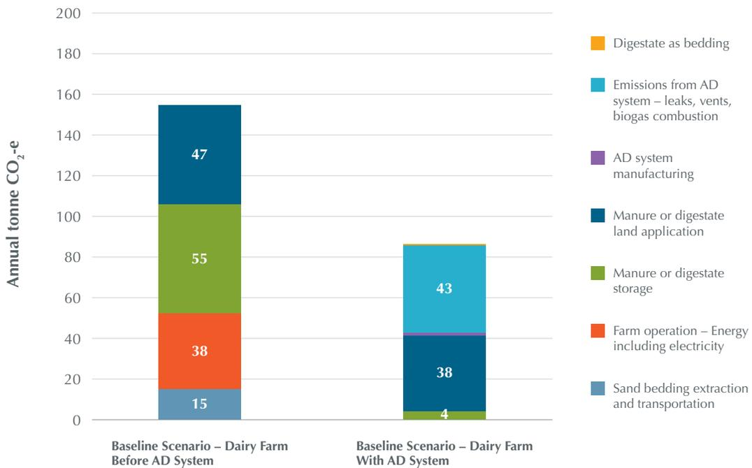
GHG quantification for the farm with and without the AD was completed. The results showed a potential annual reduction of 60 tonne CO<sub>2</sub>-e (Carbon dioxide equivalent) per system in Ontario, with potential annual additional reduction of 10 tonne CO<sub>2</sub>-e per system when including nitrous oxides (N<sub>2</sub>O) emissions from land application.
